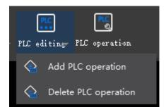
Adding PLC operations will display the required PLC actions on this page. After adding an action, the added PLC action will be displayed in the PLC operation.
