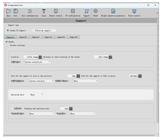
After the support function is configured in the Jinzhou CNC-configuration tool, the output port function and high and low level are set in the IO configuration. After the configuration is completed, click Save to close the configuration tool and support the debugging function in the Jinzhou CNC software. Before debugging the support function, you first need to give the Y-axis back to the origin.
