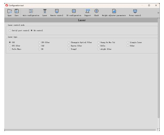
After completing the laser configuration, the power and frequency of the laser point can be set at the operating bar on the right side of the software. After setting the parameters, open the light switch and press the laser key to see if the laser is configured successfully.
