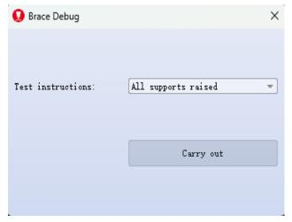
Support with the Y drop position parameter greater than the current actual Y coordinate value is considered a safe support and can be manually raised and dropped on the manual debugging page. At this point, the stopwatch can be used to measure the time of support rise and fall, and the default time and fall position parameters can be further adjusted.
