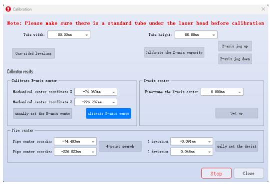
Note: Accurate and reliable coordinates of the X / Z / W axis are needed before calibrating the center of axis B; that is, before calibrating the center of axis B, all the axes of the machine should return to the origin.
