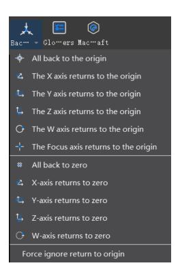
The drop-down menu of "back to the origin" contains all back to the origin, X axis back to the origin, Y axis back to the origin, Z axis (raise) back to the origin, W axis back to the origin and focal axis back to the origin, and all zero, X, Y, Z, W axis back to zero.
