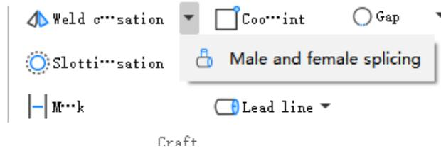
By changing the knife path, the oblique cut parts are divided into two different shapes: the male and the female, so as to realize the L-type splicing of rectangular tubes.
