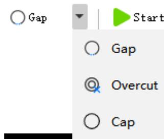
Select a drawing to click the drop-down box in the drawing to adjust whether the drawing is closed, notch, or overcut. The default drawing is the seal, which means that the end point overlap; the start and end point of the notch do not overlap. The difference is that the gap is cut less and the notch is cut more.
