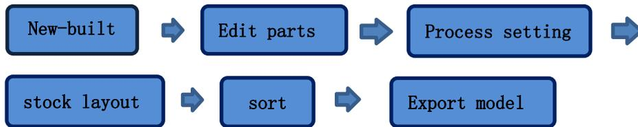
The most common use process of Jinzhou CNC 3D set material software is shown above, and the common operation steps will be demonstrated next.
