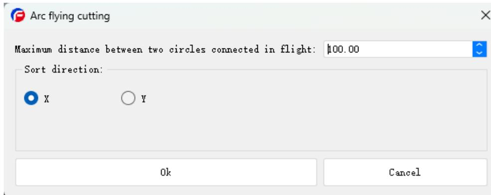
Use a circular arc to cut regularly arranged circular holes on pipes (whether circular or rectangular).
