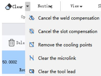
Select the track to clear the process, open the clear drop-down box to select the process to be cleared, and click to clear all the corresponding processes of the selected track.
