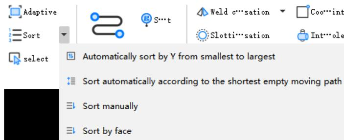
① Automatic sorting according to Y from small to large: start from the Y value near the starting section, move along the direction of the pipe to the other end of the pipe, and the order of the graph is the order of arrangement.
