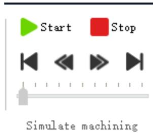
To simulate the processing of the cutting head on the pipe, you can clearly see the cutting order, direction and other information. Click Start to start cutting the current part or sample result, and if some drawings are selected, only the selected ones. In the simulation state, click "
