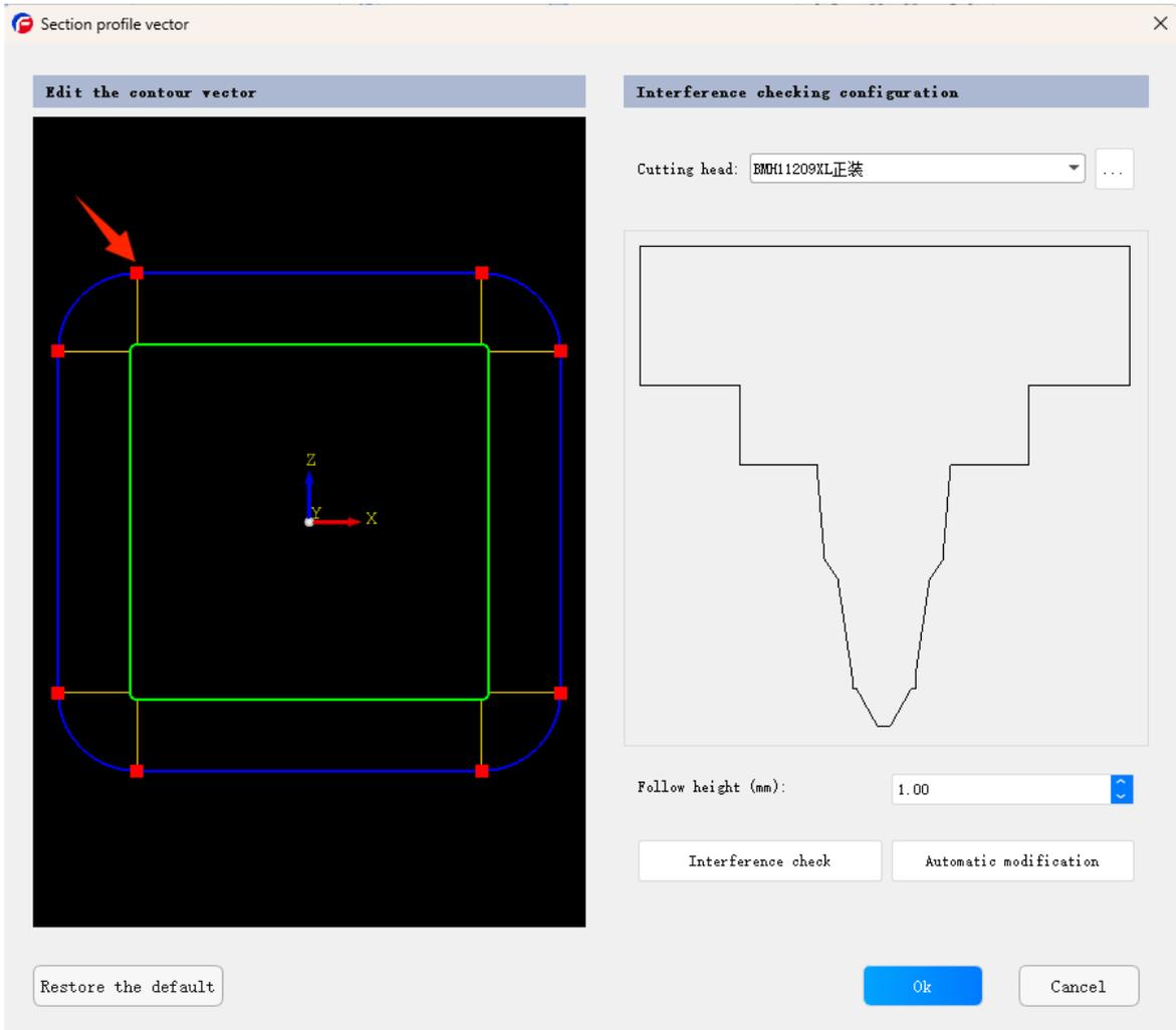
Click to edit the section profile vector, and the section normal vector can be adjusted by dragging the adjustment point. After the adjustment, click the interference check can judge whether the currently selected cutting head profile and pipe are interfered or not.
