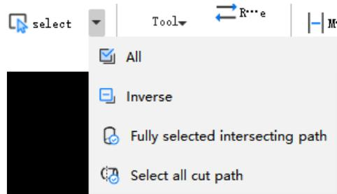
For the model displayed in the current window, click select, reverse, select consistent trajectory, and cut off trace. You can quickly select the desired track.
