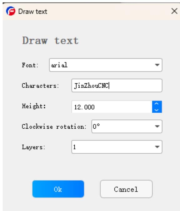
Open "Draw Text", select the font, set the text content, set the font height, font rotation direction and layer, click OK, and move the mouse to add the text where you need to draw.
